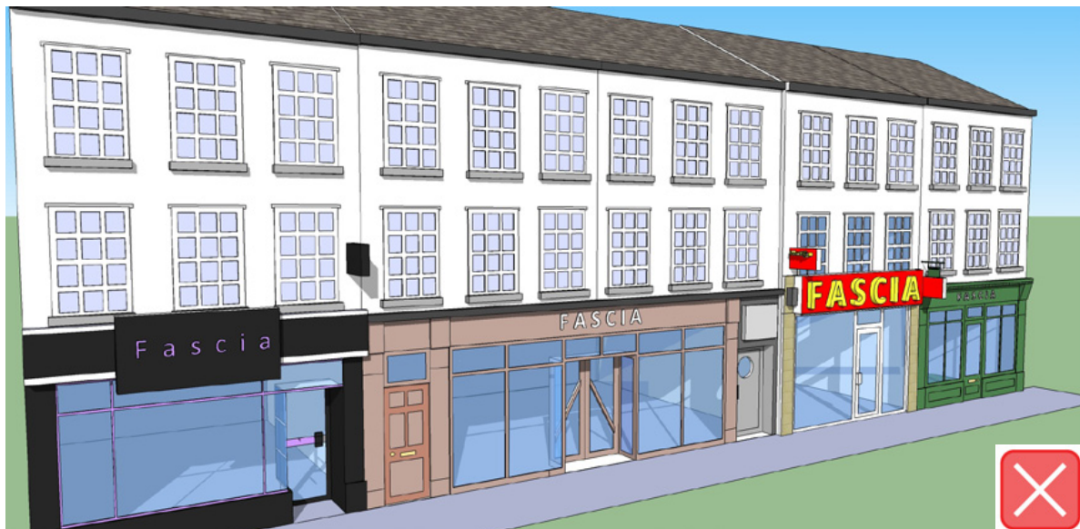
Figure 7: Rhythm of the street -The negative impacts of mixing shopfront styles without due regard for street scene. Negatives on this street include the mixture of; signage, fascias, doorways, materials and the colour palette.
